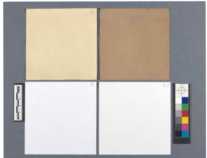
Fig. 2 Sample of yasha inpainting before (left) and after (right) climate aging (top row) and references (bottom row). (© Justine Bolle)
