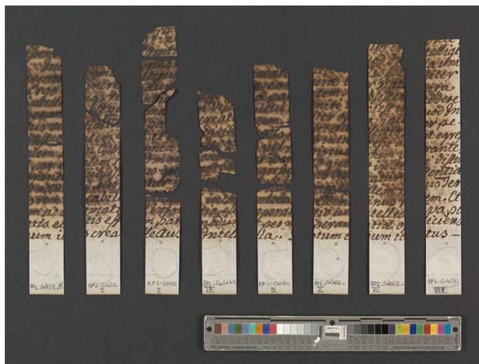
Fig. 2 Samples of historic paper with iron gall ink corrosion treated with nanolime dispersion. (© Staatsarchiv Zürich)
