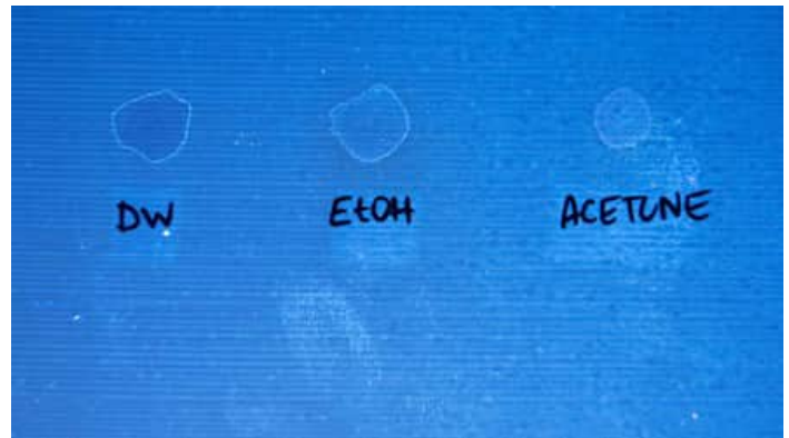
Fig. 2 Solvent spot tests on TerraSkin stone paper under ultraviolet emission. (© Restorart)
