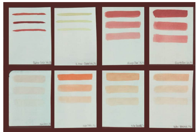
Fig. 2 MSI: NIR-false color image (940nm) of different inks on gelatine-sized paper. Top row: various iron gall inks. Bottom row: bistre and sepia inks. (© Carsten Wintermann)
