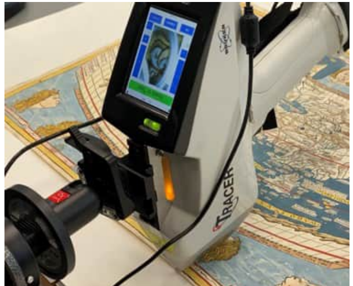
Fig. 2 XRF analysis on a 1482 map. (© National Library of Norway)
