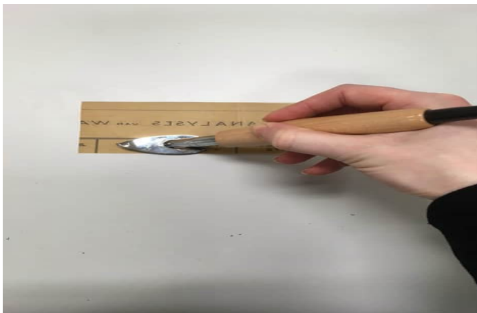
Fig. 1 Test application of a heated spatula at 120°C on a creased part of paper #1. (© M Montcalm)
