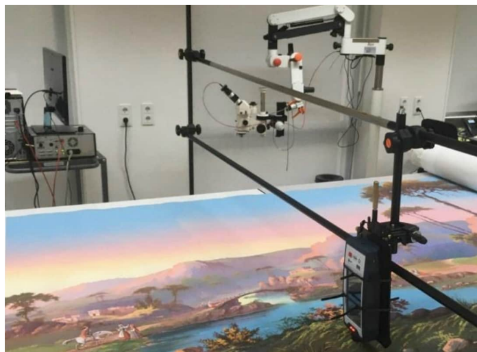
Fig. 1 Technical analysis of the colours: Raman spectroscopy_BK-18283-A. (© Femke Coevert, Rijksmuseum)
