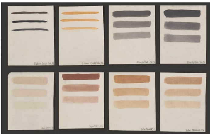
Fig. 1 VIS: Different inks applied on gelatine-sized paper. Top row: various iron gall inks. Bottom row: bistre and sepia inks. (© Carsten Wintermann)
