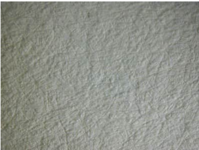
Fig. 1 Mixture of two fibre sizes, unbeaten, reemay-drying. (© Elisa Díaz)
